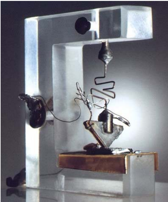
1 st transistor, Bell Lab 1947
