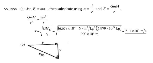
In the satellite's frame of reference, the rivet has two perpendicular velocity components equal to v from part (a):
