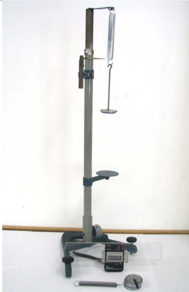
Fig. 4. Set of the experiment with Jolly balance
