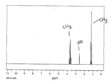
b. On the axis provided below draw what the proton NMR spectrum of an ANHYDROUS sample of ethanol would look like. Note: the alcohol H will NOT undergo exchange here and splitting WILL be observed.
