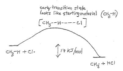
7c. In the case of CI, there is not much difference in activation energy between reacting a 1°,2° or 3° position.
