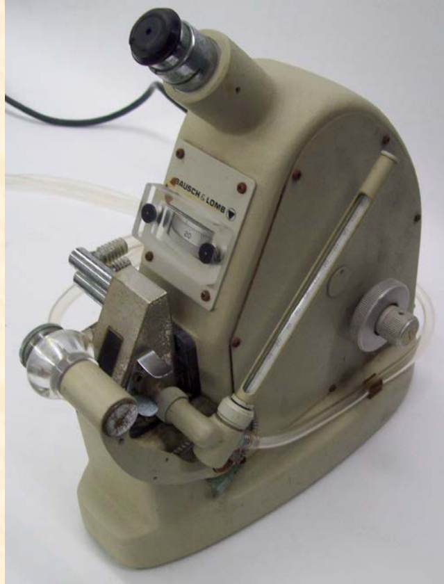
Figure 1. The Bausch and Lomb refractometer (right side view). On this instrument the compensator is a dial located on the front of the instrument (behind a protective plastic window in this view) below the eyepiece and above the sample stage. The prism coarse adjust and fine adjust knobs are the large and small knobs, respectively, located on the right side of the instrument. This instrument's light source is external and is housed in the arm on the front of the instrument which can swing down and away from the sample stage. On this instrument the power switch is at the rear.
