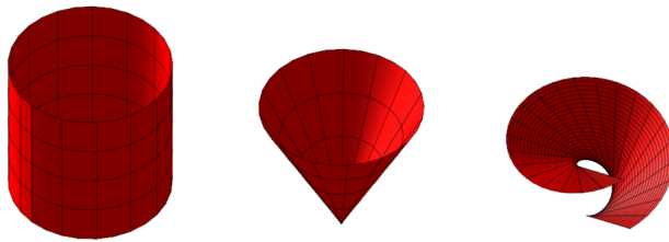
FIGURE 1.4. Three developable surfaces: although they appear curved in three-dimensional space, they can be unwrapped onto a plane, and geometers living on the surface would perceive each one as Euclidean.
